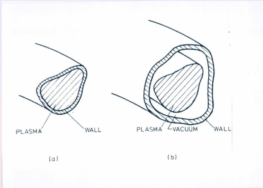
A toroidal plasma configuration: (a) surrounded by a perfectly conducting wall;
