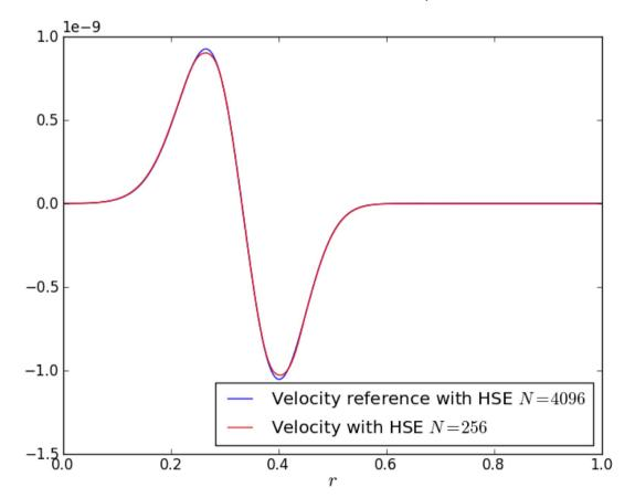
Without HSE reconstruction the velocity is way off!
